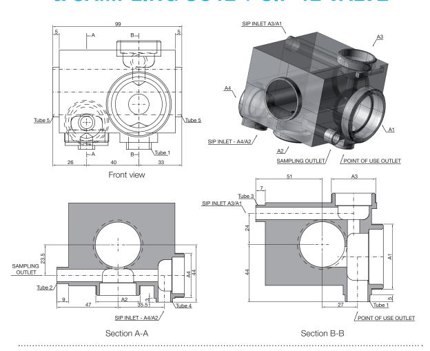
Clean and Aseptic Valves of CAD Product Line have simple and safe design, with their full drainability, without asymptotic seal and dead leg, are offering fast cleanability and sterilization practices. They are designed to fulfil stringent demands of CIP-SIP and Production Cycles on Aseptic Processing.
