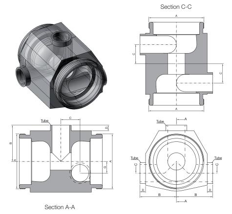
Clean and Aseptic Valves of CAD Product Line have simple and safe design, with their full drainability, without asymptotic seal and dead leg, are offering fast cleanability and sterilization practices. They are designed to fulfil stringent demands of CIP-SIP and Production Cycles on Aseptic Processing.
