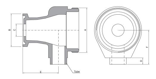
Clean and Aseptic Valves of CAD Product Line have simple and safe design, with their full drainability, without asymptotic seal and dead leg, are offering fast cleanability and sterilization practices. They are designed to fulfil stringent demands of CIP-SIP and Production Cycles on Aseptic Processing.
