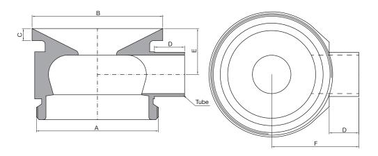
Clean and Aseptic Valves of CAD Product Line have simple and safe design, with their full drainability, without asymptotic seal and dead leg, are offering fast cleanability and sterilization practices. They are designed to fulfil stringent demands of CIP-SIP and Production Cycles on Aseptic Processing.
